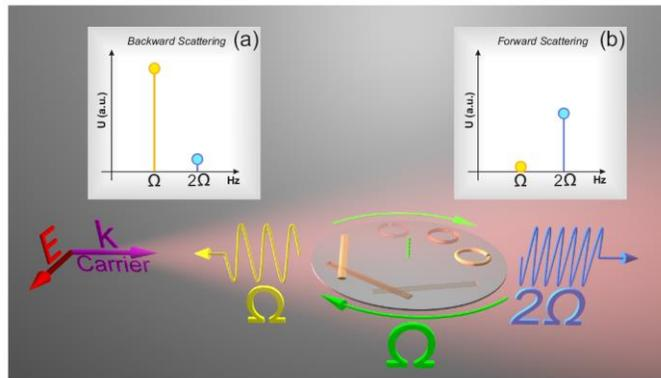
**Fig. 1.** Illustration of an asymmetric micro-Doppler comb generation from axially rotating magneto-electric particle (HMEP). Split ring resonator and a wire, forming the HMEP, are rotated with an angular frequency  $\Omega$  in the polarization plane of the incident wave. Forward and backward scattered fields demonstrate different micro-Doppler spectra (insets illustrate frequencies at the baseband).
