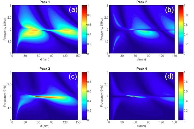
**Fig. 4.** Amplitudes of the micro-Doppler peaks in the backscattered signal from hybrid magneto-electric particles, as the function of illumination frequency (y-axis) and separation distance between the constitutive elements (x-axis). (a) first, (b) second, (c) third, (d) fourth peaks in the comb. All the color maps are normalized to the same value.
