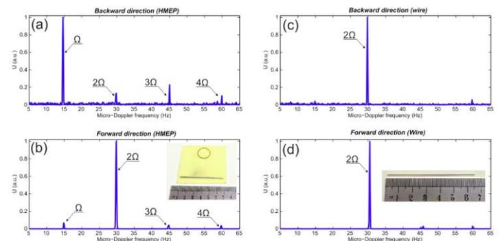
**Fig. 6.** Experimental observation of micro-Doppler combs. (a, b) – HMEP particle; (c,d) – thin metal wire. Upper row – backward direction, lower row – forward direction. Angular frequency of mechanical rotation is  $\Omega = 2\pi \times 14 \text{ Hz}$ . Insets – photographs of the samples.
