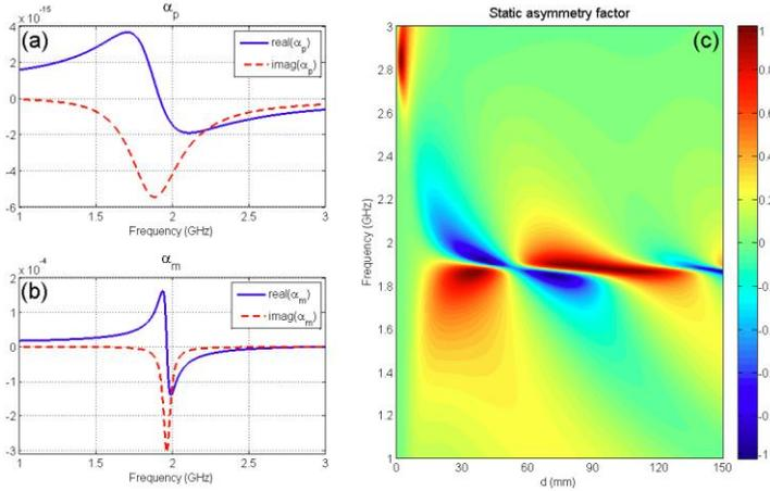
**Fig. 3.** Properties of the static configuration. (a) polarizability of the wire, as the function of frequency. (b) polarizability of the split ring, as the function of frequency. (c) color map of the static asymmetry factor, as the function of frequency (y-axis) and separation distance between the wire and the ring (x-axis).
