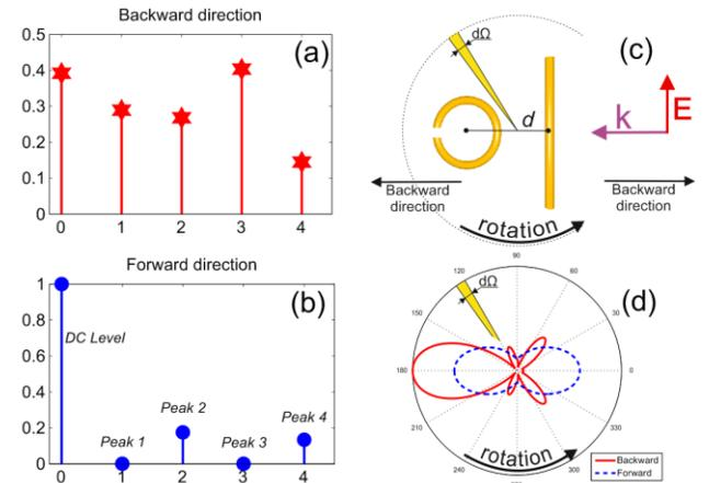
**Fig. 2.** Nonlinear frequencies generation by axially rotating magneto-electric particle (HMEP) – analytic theory. Micro-Doppler frequency comb in backward (a) and forward (b) directions. Particle parameters are  $d = 38 \text{ mm}$ ,  $R_{SRR} = 9.5\text{mm}$ ,  $L_{Wire} = 60\text{mm}$ , the illumination frequency is
