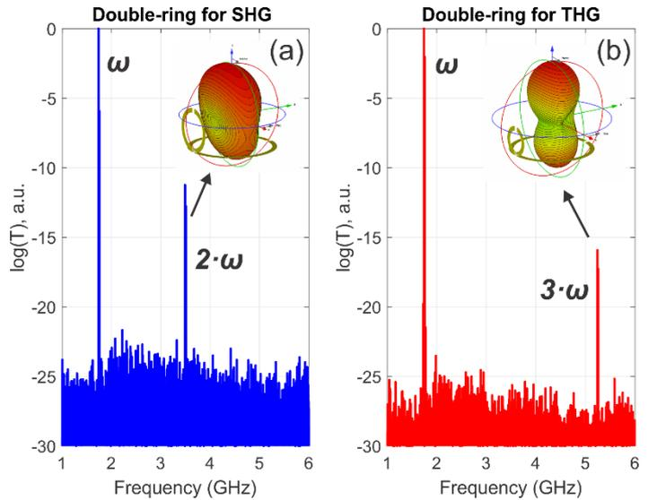
**Fig 5. (Color Online).** The near-to-far field transmission (experimental data on the logarithmic scale) for the double-ring optimized for SHG (a), and THG (b). In both cases, the transmission at the pump frequency is normalized to unity. Insets display far-field radiation patterns.
