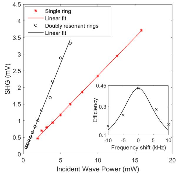
Fig 3. (Color Online). The second-harmonic generation efficiency in the near-to-near field configuration, as a function of the incident power, at  $f = 1.737$  GHz. Dots – experimental data, lines – a linear fit to them. The insert shows the SHG efficiency as a function of the pump-frequency detuning (in KHz) from the central resonant frequency.
