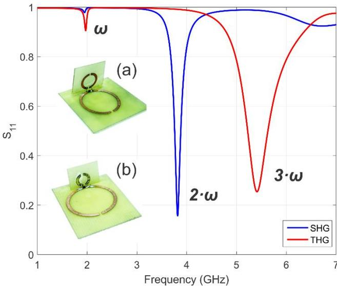
Fig 2. (Color Online). Reflection amplitudes (the absolute values of the  $S_{11}$  parameters) of the double-rings setting (numerical data), tuned for second-harmonic or third-harmonic generation (blue and red lines, respectively). Insets are photographs of the fabricated samples: (a) for SHG, (b) for THG.
