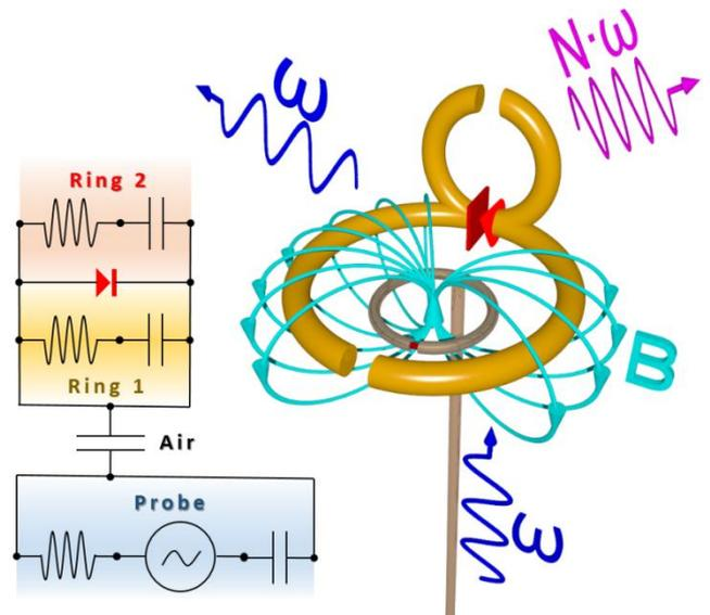
Fig 1. (Color Online) Schematics of the doubly-resonant nonlinear meta-atom, built as a pair of split-ring resonators sharing a varactor diode at a joint gap. The grey loop underneath the lower ring is an excitation probe. The left inset displays a lumped circuit scheme of the system.
