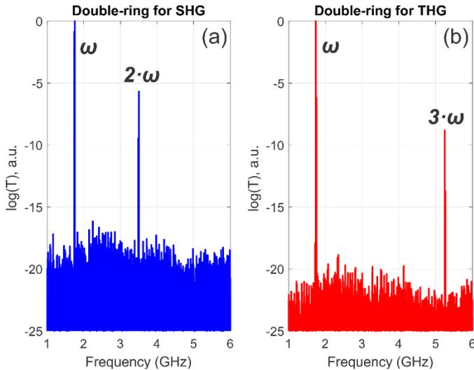
**Fig 4. (Color Online).** The near-to-near field transmission (experimental data on the logarithmic scale) for the double ring optimized for SHG (a), and THG (b). In both cases, the transmission at the pump frequency is normalized to unity.
