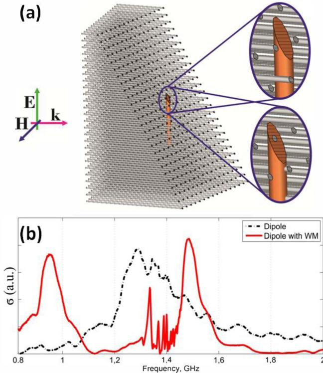
Fig. 1. (a) Schematic layout of the experimental sample. Insets underline two types of interaction regimes – ‘contact’ (lower inset) and ‘non contact’ (upper inset). (b) Experimental radar cross-sections (arb. units). Red solid line – 100 mm dipole in 200 mm metamaterial, black dot-dashed line – the same dipole in the free space. The parameters of the wire medium are - 17x26 array of thin metal wires, with diameters equal to 2 mm and length – to 200 mm.
