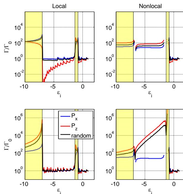
Fig.5 Emission of the point dipole positioned in the vacuum slit inside the lossless nanowire metamaterial; top and bottom rows correspond, respectively, to results of calculations that are not and are accounted for local field corrections
