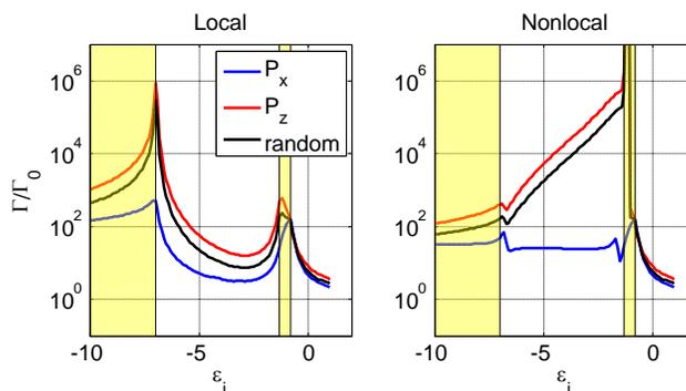
Fig.6 Enhancement of decay rate in metamaterials with finite lossess; the plots take into account local field correction;  $Im(\epsilon_i) = 0.1$ ; see Fig.1 for effective medium parameters
