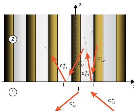
Fig.3 Schematic of light reflection and transmission at the interface between local and nonlocal media
