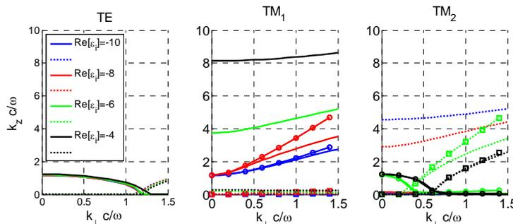
Fig.2 Dispersion of the three waves supported by metamaterial for different permittivities of the nanowires: (solid line)  $Re[k_z c/\omega]$ , (dashed line)  $Im[k_z c/\omega]$ , (symbols) dispersion of “main” TM-polarized mode according to local EMT. All other parameters as in Fig. 1.
