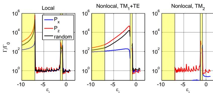
Fig. 4 Enhancement of decay rate in infinite lossless metamaterials (lines of different colours represent different orientation of the dipole);
